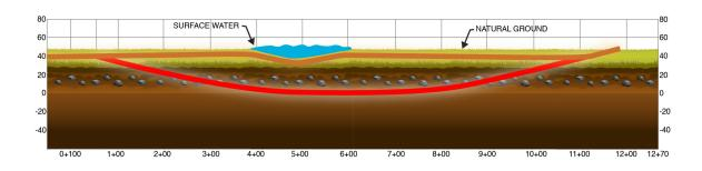
This drilling technique will be used at the onshore and inshore areas of the project along the Port Aransas Causeway on Highway 361, across the Intracoastal Waterway, and is planned for both Aransas Pass Channel and Lydia Ann Channel (see map on opposite side).
